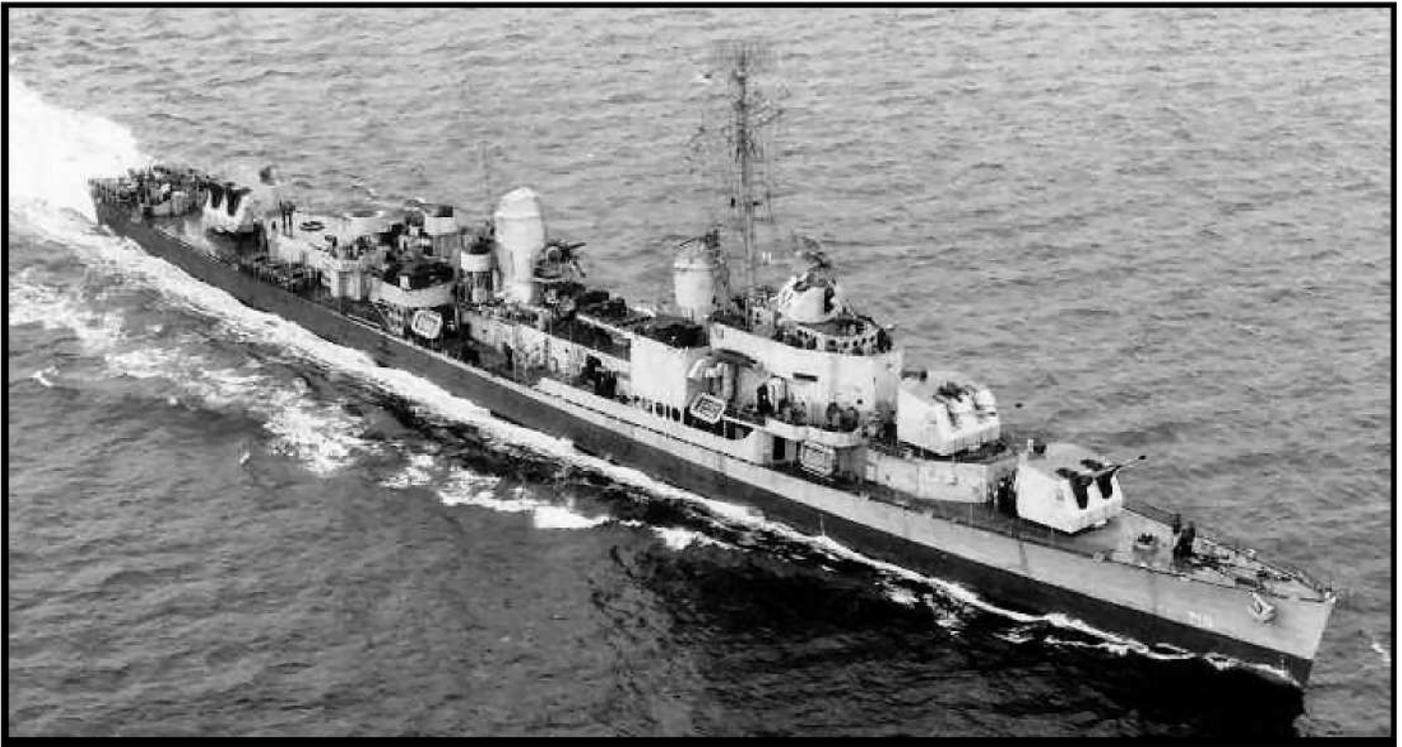
Gearing after the torpedo tubes were removed (Not the ring where they were)
